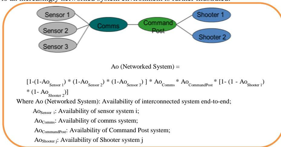
**Fig. 2.** Analytical computation for simple networked system availability
